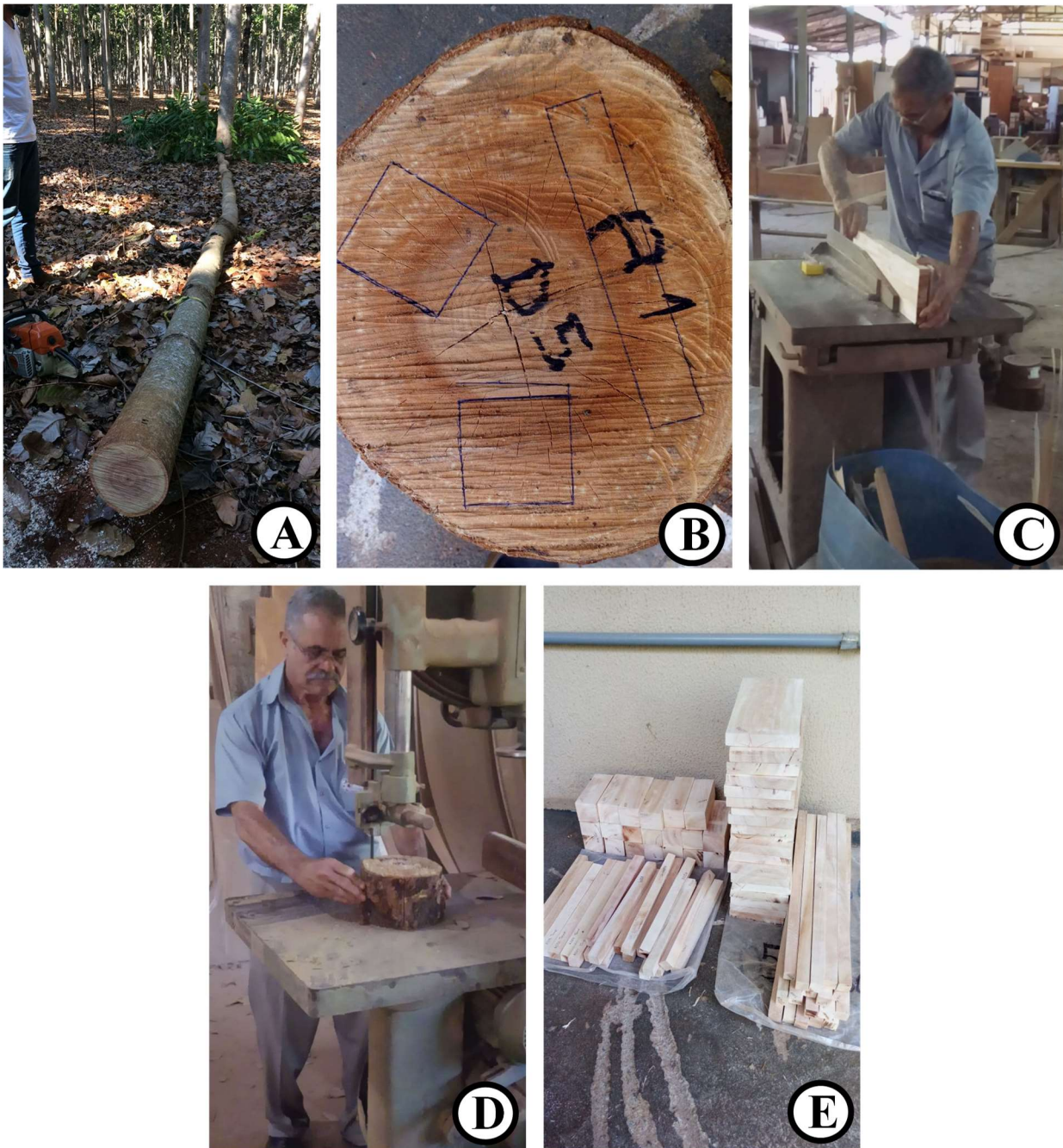
Appendix 1. Sampling and preparation of wood samples of Khaya sp. trees. A: Wood discs and log sampling; B: Samples identification and demarcation; C and D: Wood samples preparation and E: Wood samples read for tests.
