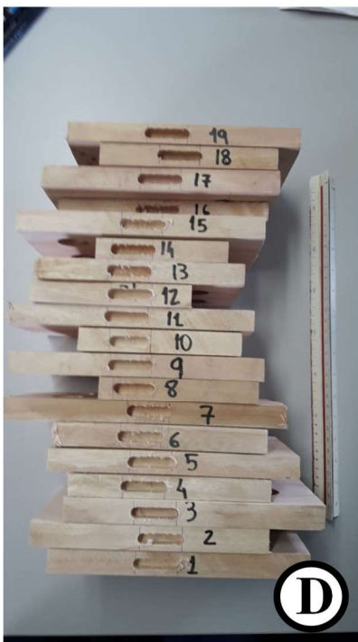
Appendix 3. Machining tests in Khaya sp. wood samples. A: Surfacing; B: Boring; C: Sanding; D: Mortising; E: Nail splitting and F: Abrasive wear resistance
