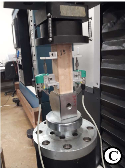
Appendix 2. Physical and mechanical tests in Khaya sp wood samples. A: Specific gravity and shrinkage; B: Impact bending; C: Compressive strength parallel to grain; D and E: Turing.
