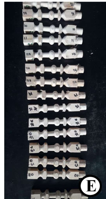
Appendix 2. Physical and mechanical tests in Khaya sp wood samples. A: Specific gravity and shrinkage; B: Impact bending; C: Compressive strength parallel to grain; D and E: Turing.
