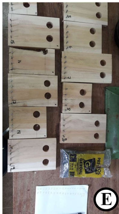
Appendix 3. Machining tests in Khaya sp. wood samples. A: Surfacing; B: Boring; C: Sanding; D: Mortising; E: Nail splitting and F: Abrasive wear resistance
